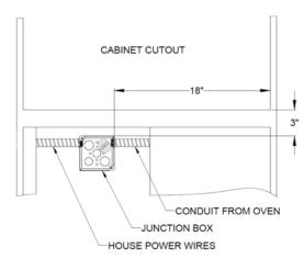
Move the oven with flexible conduit/wires close to the cabinet cutout and feed the wires and conduit through the rectangular cutout located at the rear end of the cabinet cutout base
